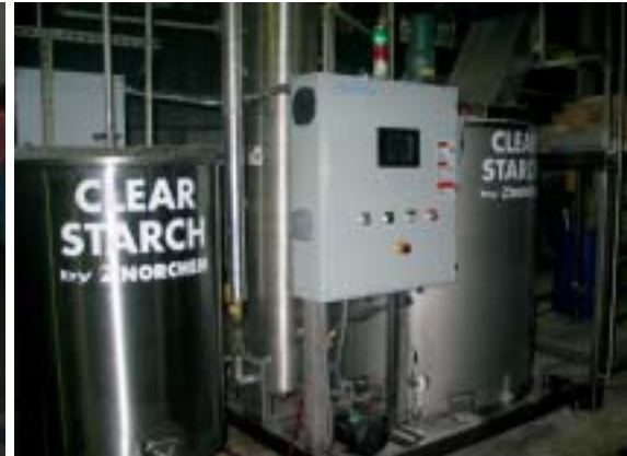
Mission utilizes the Norchem Starch Cooker to improve the finish on table linens.
