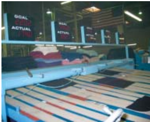
The plant has three, wide-lane ironers, which are both fitted with production-monitoring display screens that show current production against the day's goals.
