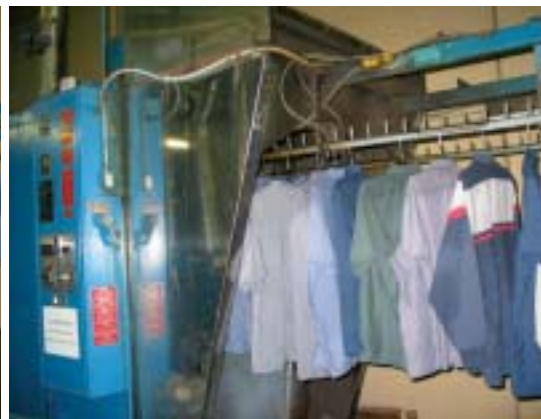
After industrial items are washed and dried, they are placed on hangers and make their way into the plant's Colmac tunnel finisher. Garments also are finished on Colmac's Triple Connie and Unipress' coat press.
