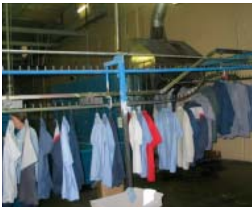
After industrial items are washed and dried, they are placed on hangers and make their way into the plant's Colmac tunnel finisher. Garments also are finished on Colmac's Triple Connie and Unipress' coat press.
