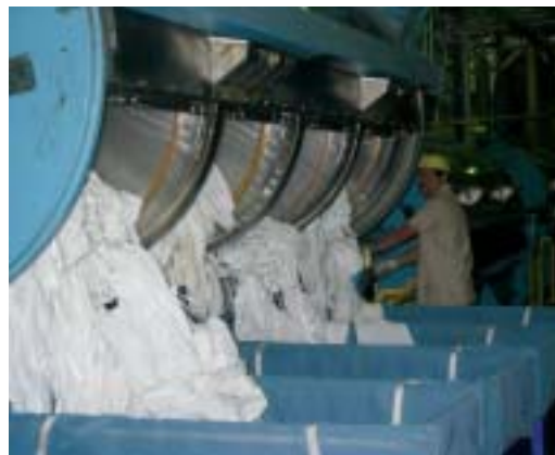
The four-pocket Ellis washers unload food and beverage items into laundry carts. Mission employees are trained to think safety first as they move goods through the wash aisle.
