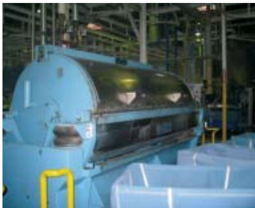
The plant uses seven washers in its conventional wash aisle, three four-pocket Ellis machines and four 450 lb. Lavatec washers.
