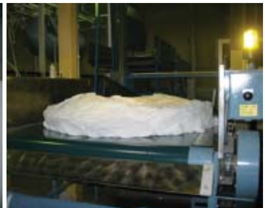
A 200 lb. cake of hospitality linen moves out of the 18-pocket Senking tunnel and awaits the shuttle to transfer it to the dryers.
