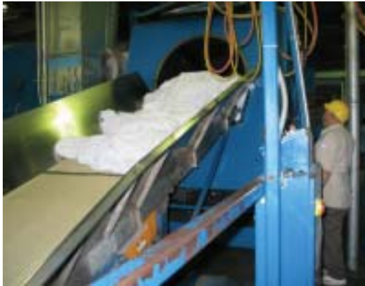
Items are loaded by conveyor system into one of five Consolidated Laundry Machinery (CLM) 400 lb. dryers used on the industrial side of the plant.
